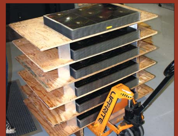
The covers had to be stacked on short lifts to ensure proper drying without distortion.
