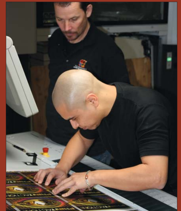
Prepress Manager Pablo Verdugo (foreground) and Lead Press Operator Mic Tomkins inspect the registration on the pieces during its run.
